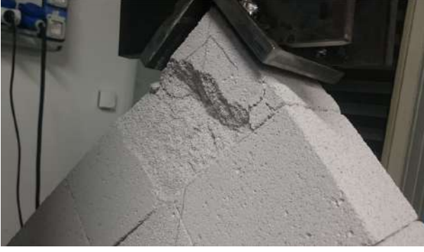
Figure 14 Scaled loading shoe; splitting failure of the corner.
