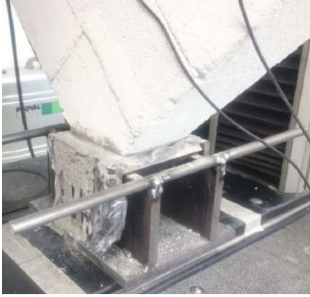
Figure 15 Closed loading shoes, filled with capping material.
