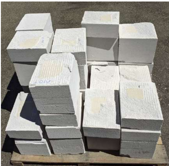
Figure 9 Shear failure in the joint, triplets assembled with PM-TLM.
