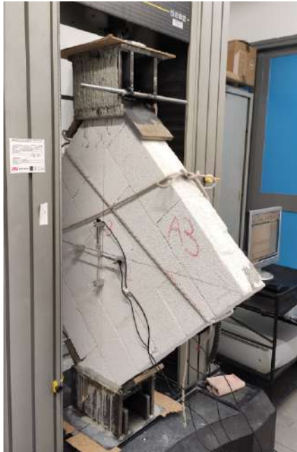
Figure 16 General view of the experimental setup adopted for diagonal compression tests.
