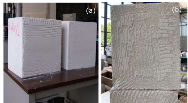
Figure 11 Shear failure in the joint, triplets assembled with AA-TLM (a) without and (b) with preliminary surface cleaning with an electric air blowing.
