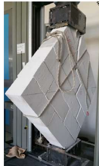
Figure 18 Stepwise diagonal crack pattern in mortar joints.
