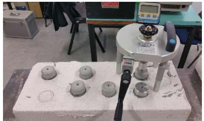
Figure 3 Experimental setup for the determination of mortar adhesive strength at 28 days.
