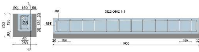
Figure 8 Geometric features of specimen AAC-RC-3 and reinforcement layout (dimensions in mm).
