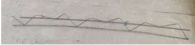
Figure 9 Lattice girder reinforcement used for specimens AAC-RC-1 and AAC-RC-2.
