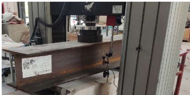
Figure 12 Detail of the LVDT applied at midspan.
