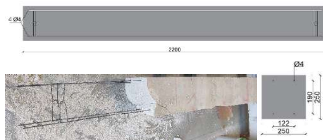
Figure 1 Geometric features of specimen AAC 25x25-1 and reinforcement layout (dimensions in mm).
