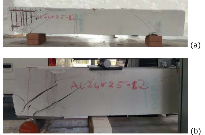
Figure 17 Crack pattern at failure for precast specimen AAC 24x25-2: (a) general view; (b) detail of the support region just before the detachment of AAC cover.
