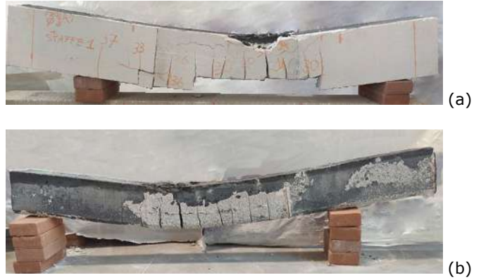
Figure 21 Crack pattern at failure for combined specimen AAC-RC-3: (a) with AAC covering; (b) after the removal of AAC covering.
