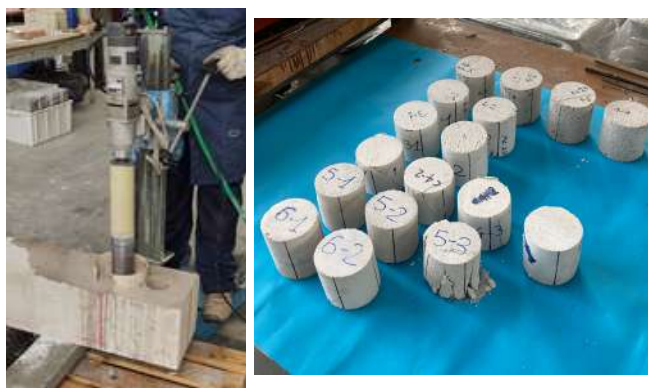
Figure 13 AAC cores extracted from precast lintels after bending test execution.
