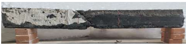
Figure 20 Specimen AAC-RC-2: (a) detail of the opening of the joint between U-shaped AAC blocks during the test; (b) detachment of AAC cover at the end of the test; (c) crack pattern at failure after the removal of the external AAC cover.
