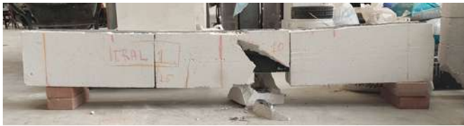
Figure 19 Crack pattern at failure for specimen AAC-RC-1.
